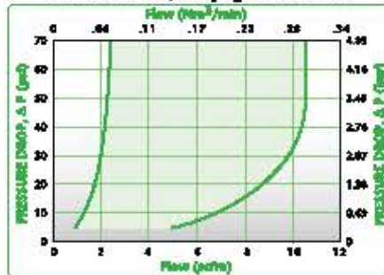
Sixtube Air Flow, 100 psig Inlet Pressure
